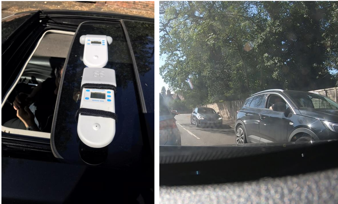
Figure 4: The two devices on the top of the vehicle to monitor air quality in the main road.
