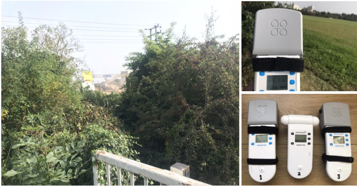
Figure 6: Three air quality monitoring devices used at an existing Quarry.
