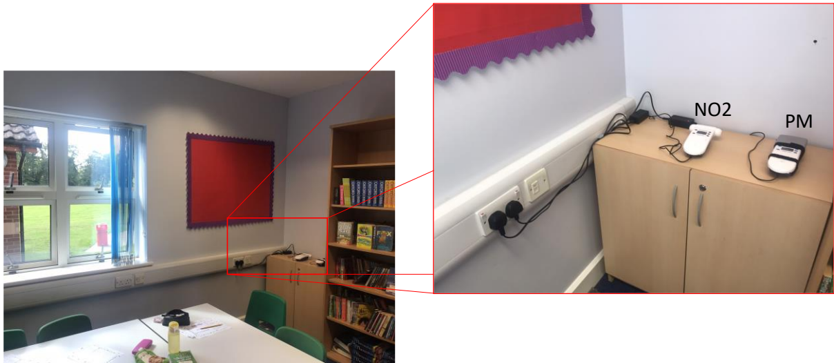
Figure 3: Two Particulate Matter (PM10 & PM2.5) and NO2 monitoring devices in the school.
