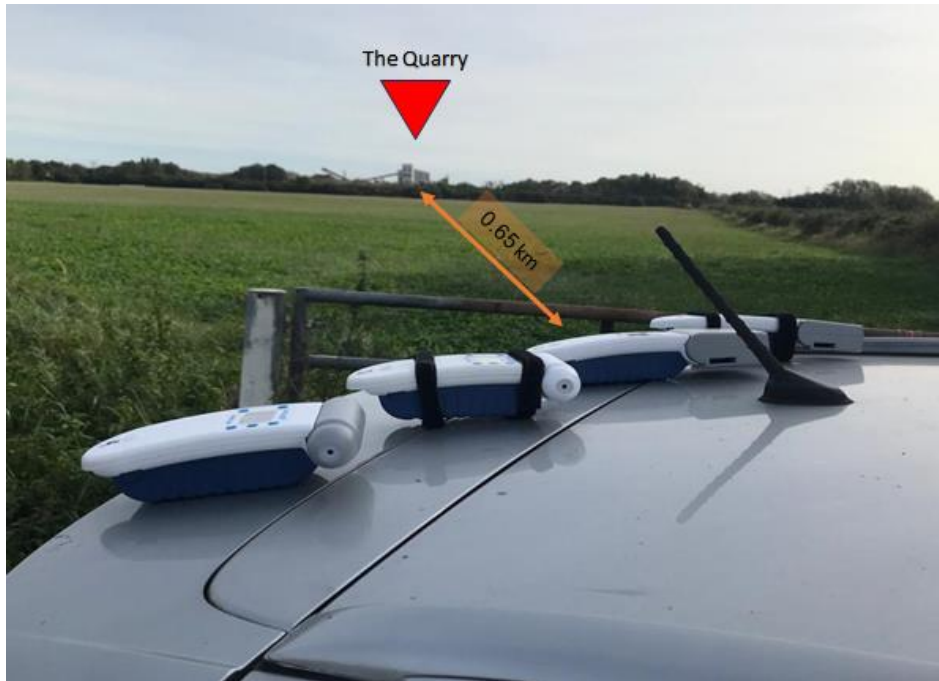
Figure 30: The four-monitoring devices in operation at the fixed point.
